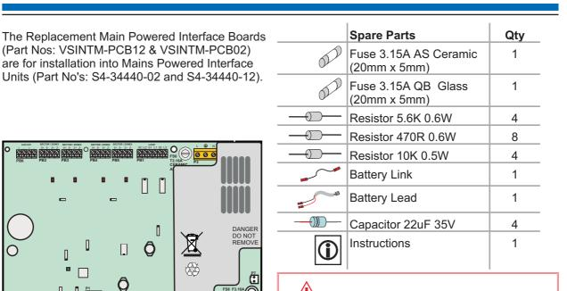
Before removal of the existing board from the Mains Powered Interface Unit first completely isolate the mains power supply to the Unit.
