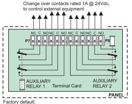
Aux relay 1 is normally de-energised and operates with a fire event without delay.
