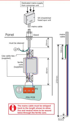
The fused spur isolator cover should be marked: FIRE ALARM - DO NOT SWITCH OFF
