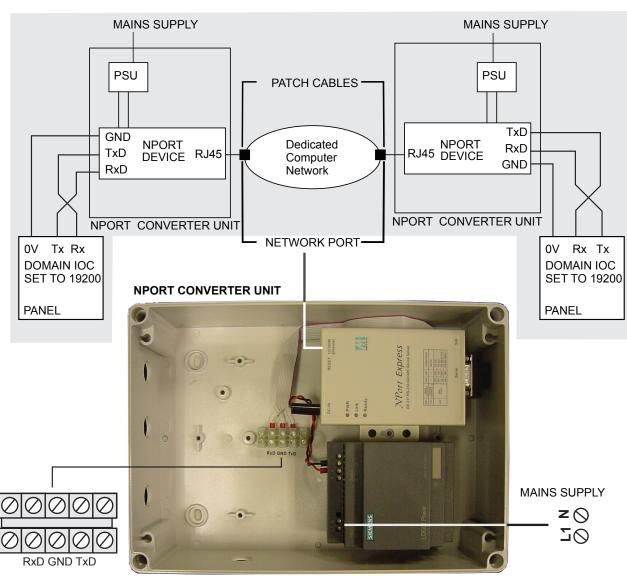
PARTS REQUIRED FOR EN54 SETUP 2 x VIG-IO-DOM 2 x VIG-NPORT-100
