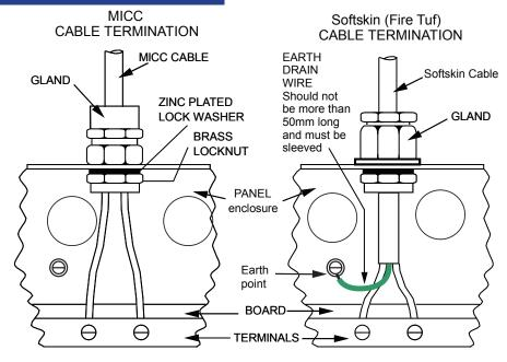
The wire length between the cable termination and point of connection must be as short as possible. Cable earth drain wire, where applicable, must be connected to the nearest earth point.
